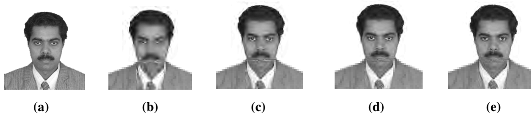
Figure 5. (a) original image (b) reconstructed image with bpp 0.1 (c) with bpp 0.2 (d) with bpp 0.3 (e) with bpp 0.4
