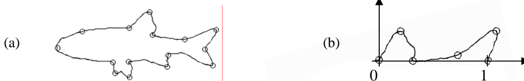
Figure 1. (a) Key points are positive local maxima and negative local minima of curvature. (b) An example of a normalized part (from front of dorsal fin to center notch of tail).
