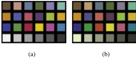
Fig. 8. Comparison (a) reproduction image of Macbeth colorchecker transformed by camera set the white balance point to W_A and (b) reproduction image considering HVS about the object.
